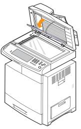
4 Remove the paper from the feed area by carefully pulling.
